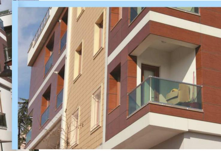
E N wall covered by composit panels and stone, aluminium glass balustrade with aluminium top rail,
